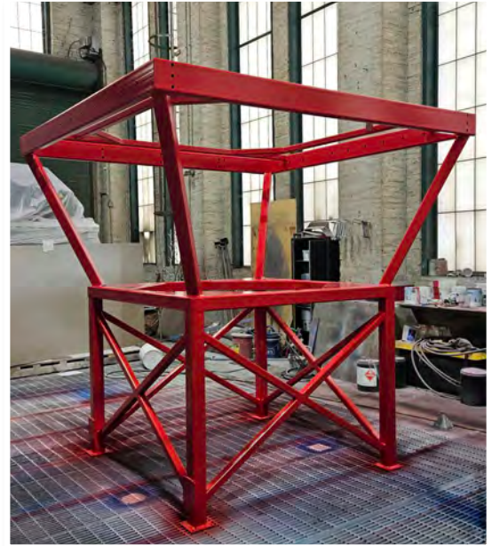
CV frame painted for customer's red zone.
