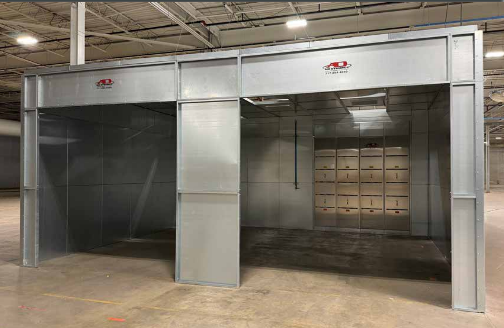
Air Dynamics' sanding booth with source capture ActiveWall dust collector.
