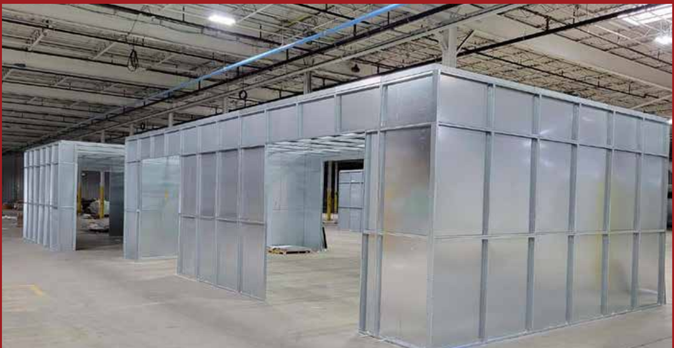
Air Dynamics' sanding booth with source capture ActiveWall dust collector.
